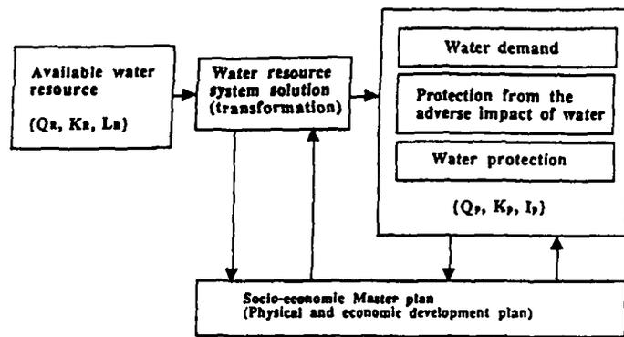
FIG. 2. Objective of Water-Resources Master Plan
