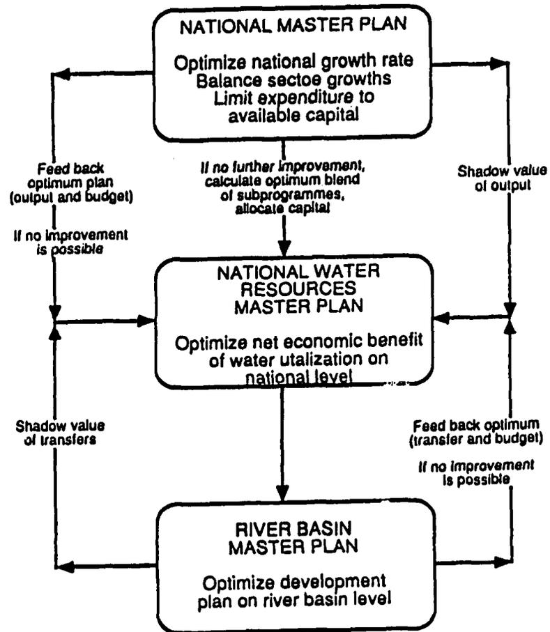
FIG. 1. Flow Diagram of Three-Level Interactive Planning System (after Haimes 1977)
