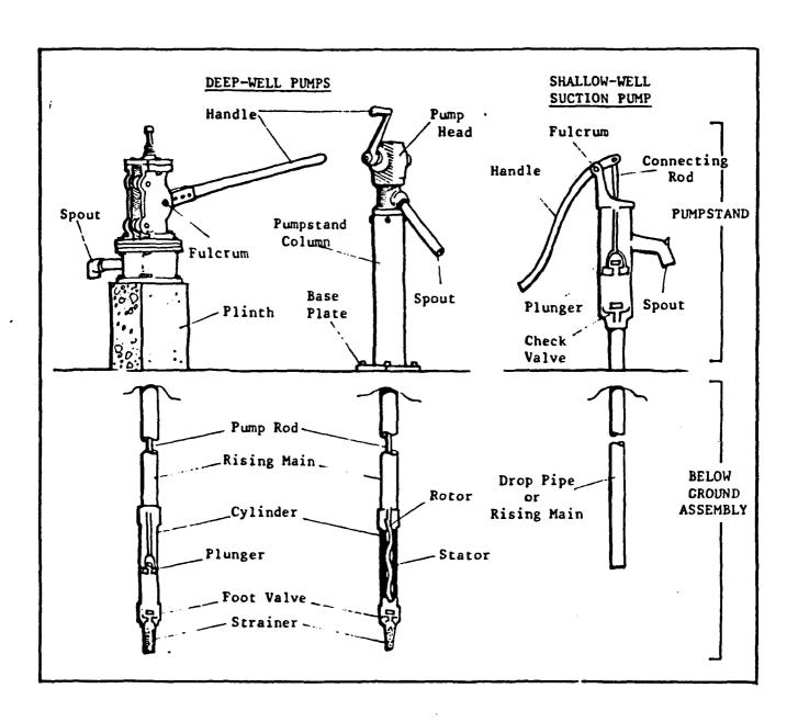
A shallow-well suction pump is one where the plunger is in the body of the pump, above ground. For practical purposes, the maximum operating depth of this type of pump is 7 metres.
