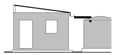
This diagram shows how a rainwater catchment system can work on a house using a Ferro cement tank or a Jo Jo.
