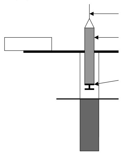
Almost any pipes can be used, as long as one fits easily inside the other. A local welder can make the flap valve and the hook for the lifting rope.
