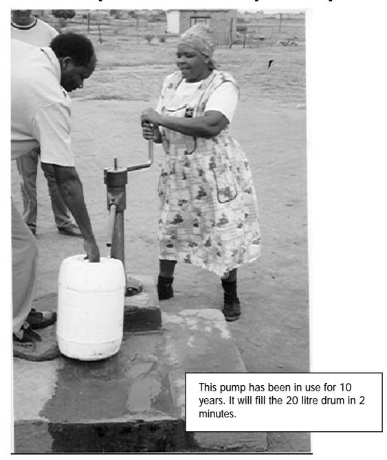
A hand pump or foot pump uses human power to lift water in a borehole up to the surface. There are many types of hand and foot pumps used in the world, and they are very simple to operate. Maintenance is very simple and spare parts are cheap, or can be made by the users. A properly installed hand pump will last for more than 20 years.
