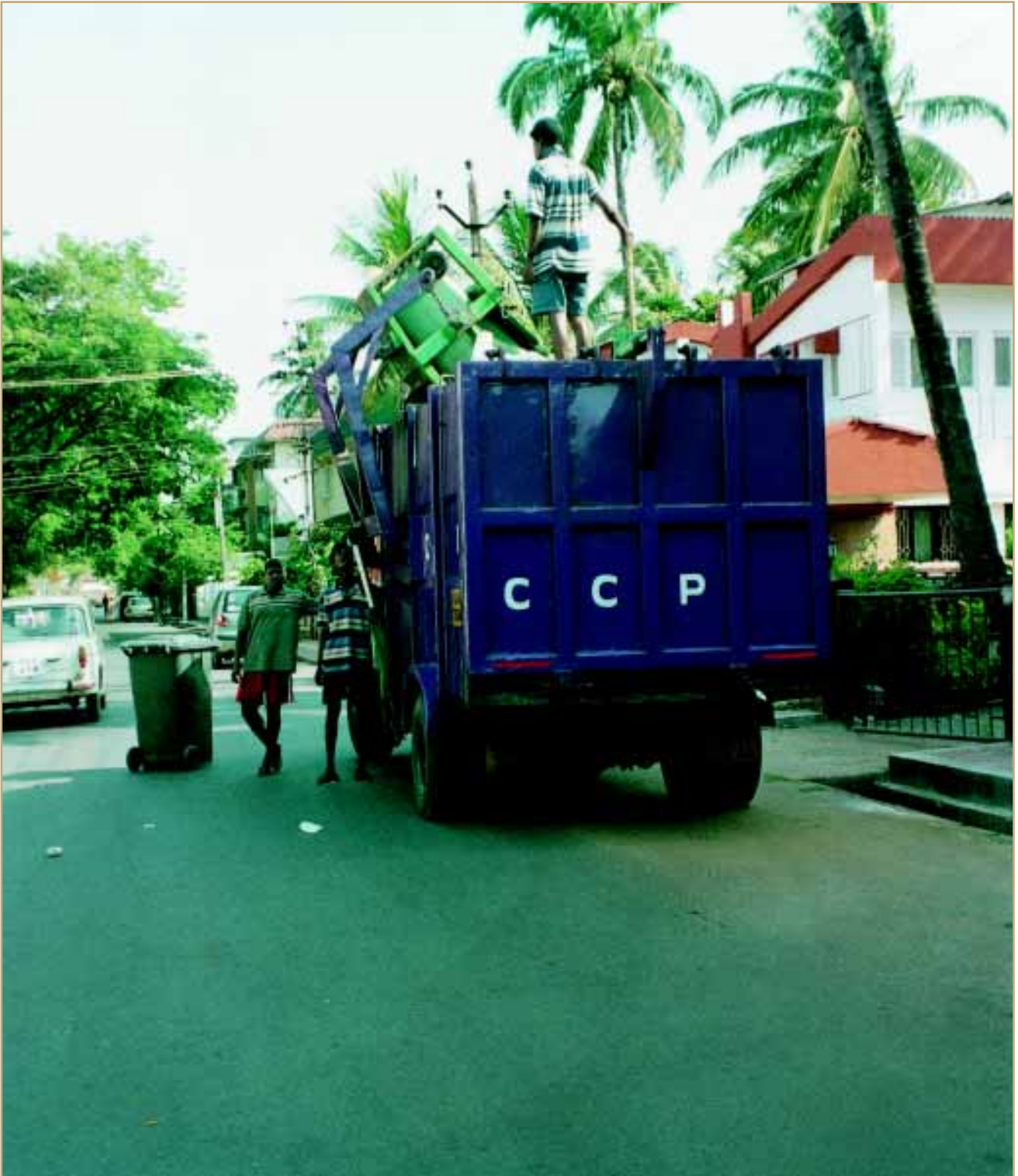
Panaji: Transfer of waste from trolley bins into trucks using a mechanized side loader.
