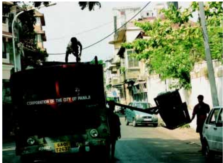
Panaji: Transfer of waste from trolley bins into trucks using a mechanized side loader.
