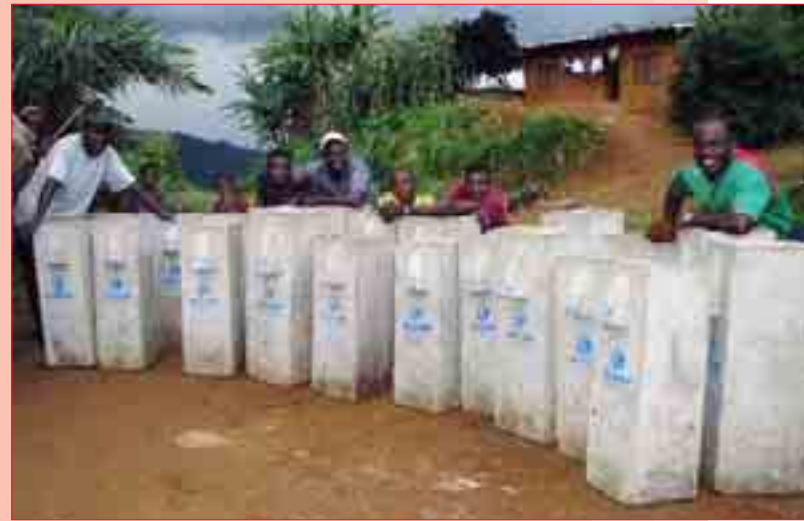
Biosand filters ready for installation at the Life Water Development Group facility in Cameroon
