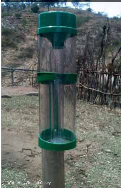
A rain gauge for monitoring rainfall installed in a village in drought-prone Konso, Ethiopia.
