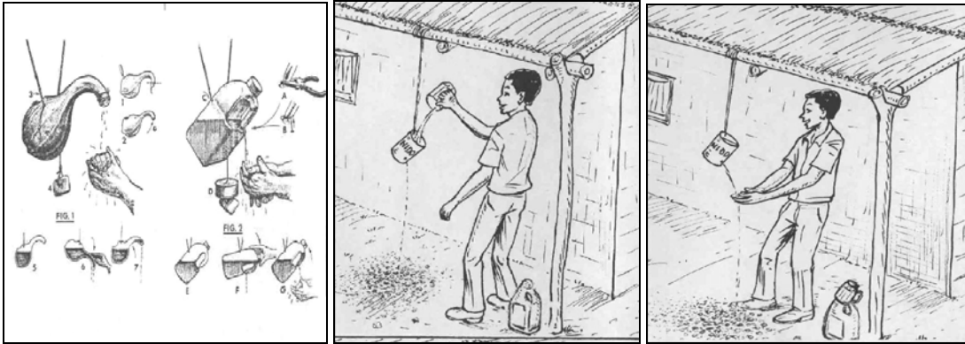
Tippy Taps: Made from a calabash and plastic bottle (Salubritas 9:4) and from an empty tin can (for SANRU [DRC] by M. Pongo).
