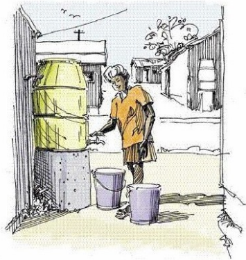
Figure 3.5. Individual yard connection with ground tank
