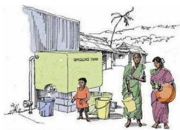
Figure 3.7. Communal yard connections with raised or ground tank
