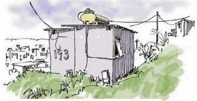
Figure 3.3. Individual house connections - daily filled overhead tank
