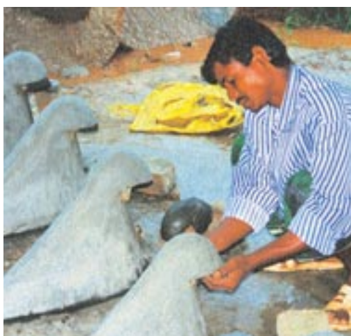
Small enterprise, producing latrine components (water seals) in Bangladesh: an effective partner for a sanitation revolution
