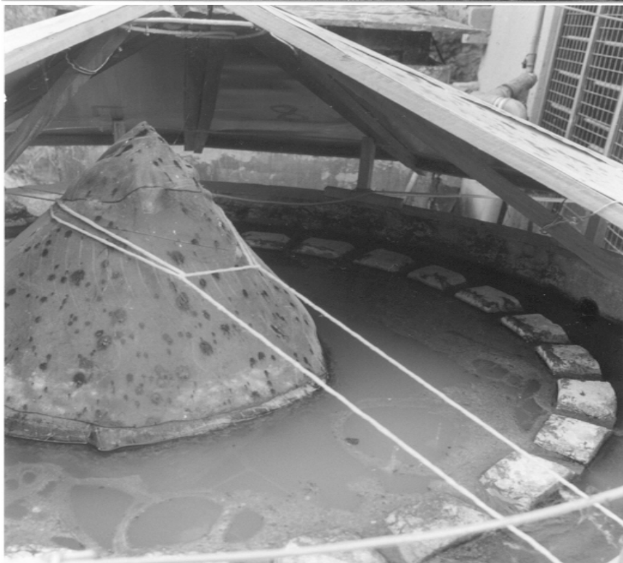
Figure 6.1b: Pilot two-step UASB reactor configuration. (a), 2m tall 1.8m 3 UASB reactor; (b), 1m tall 0.85m 3 UASB reactor.
