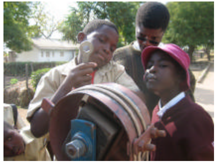
A large spanner is used to secure the nuts on the pump head
