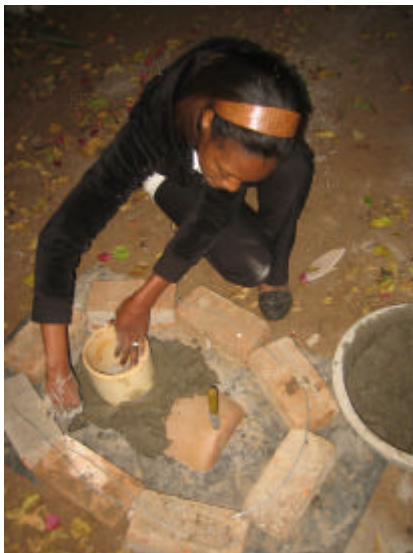
The pipe connector held in place. Concrete mix being added to mould.
