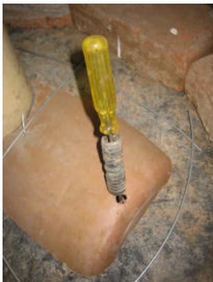
The pipe connector held in place. Concrete mix being added to mould.
