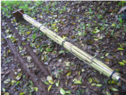
Stout tubes can be made with reeds. A fly screen is bound to the end of the tube either before or after applying the material.
