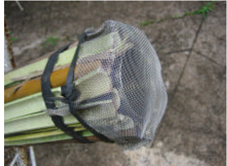
Stout tubes can be made with reeds. A fly screen is bound to the end of the tube either before or after applying the material.
