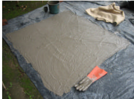
The cement paint is thoroughly applied to the first sheet using rubber gloves.
