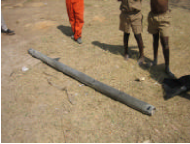
The pipe after curing. Removing the folded plastic sheet
