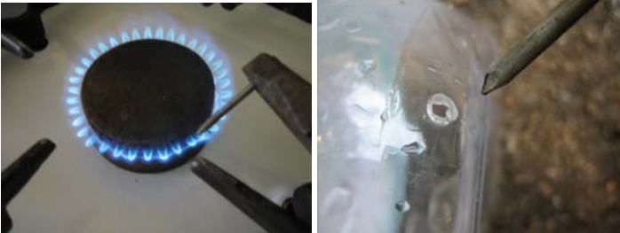
Heat the nail with a flame and carefully push into the base of the bottle
