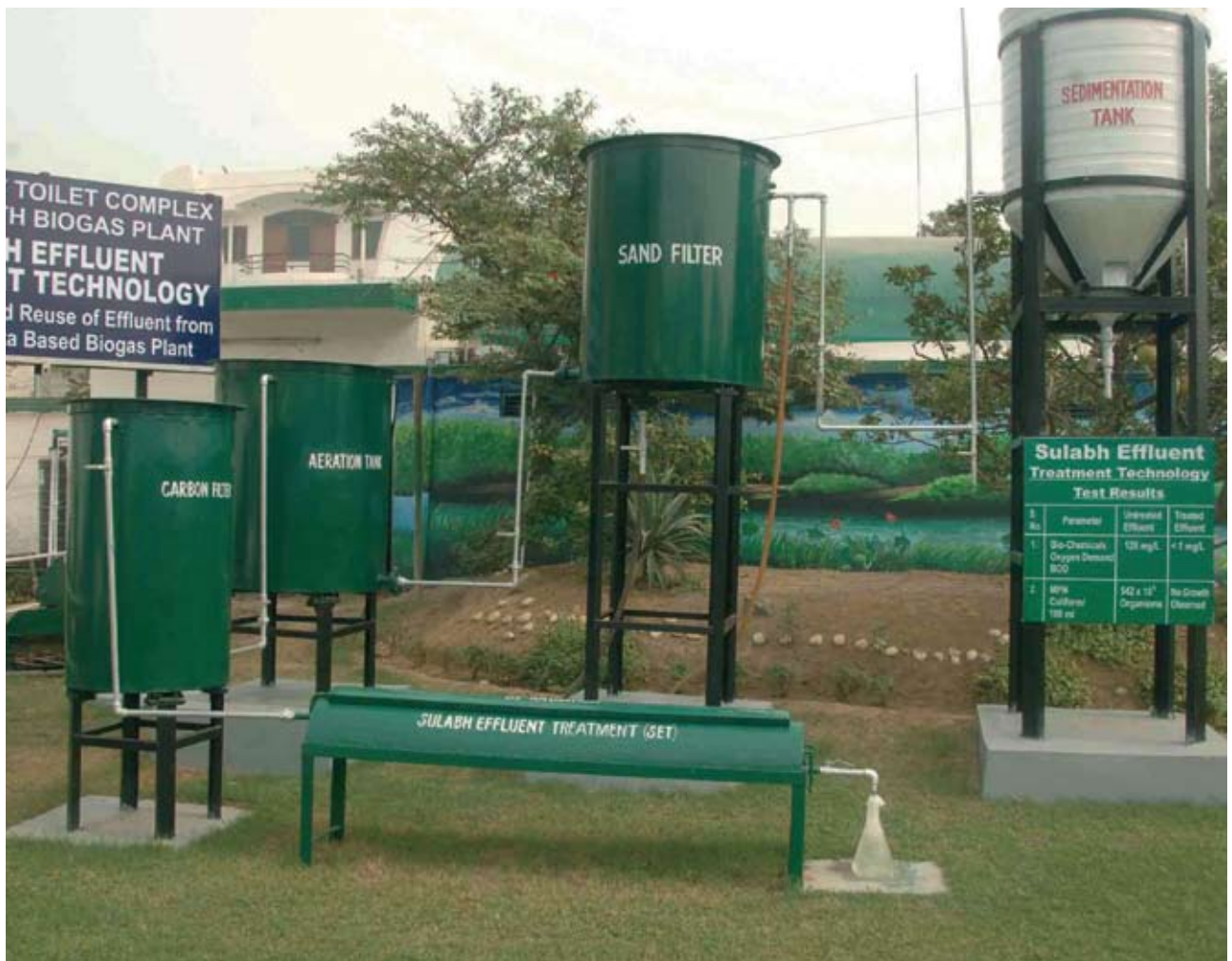
Figure 6. Sulabh Effluent Treatment (SET) technology
