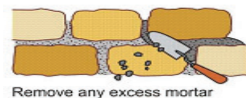
Figure.3.5 Removing of any excess mortar
