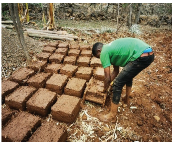
Figure: 2.1. Mud block production
