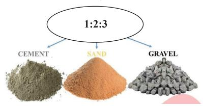
The general formula for quantizing concrete making materials is given below. You can use this formula for more calculation over any concrete of your need.
