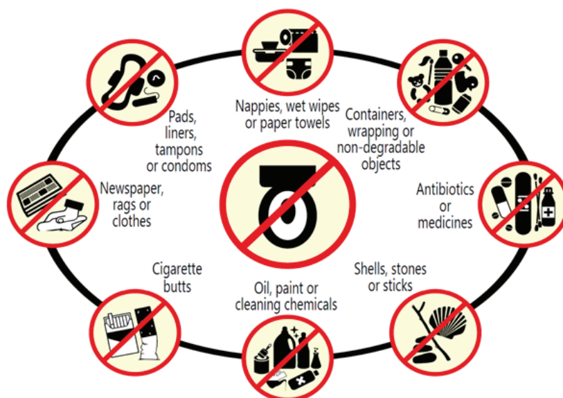
Figure 3: Examples of Items not to be thrown in latrine pits.
