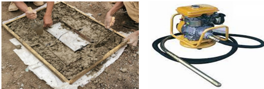
Fig-26: Hand and mechanical compaction
