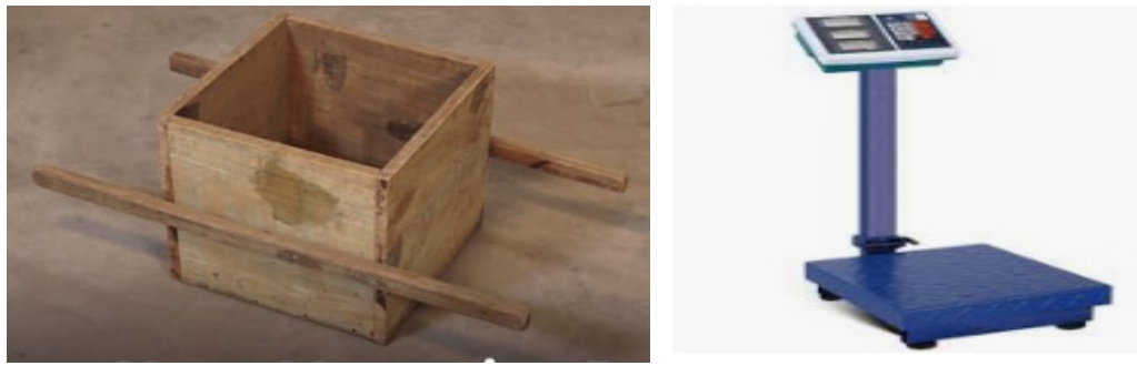
Fig-21: Volumes and weight batching.
