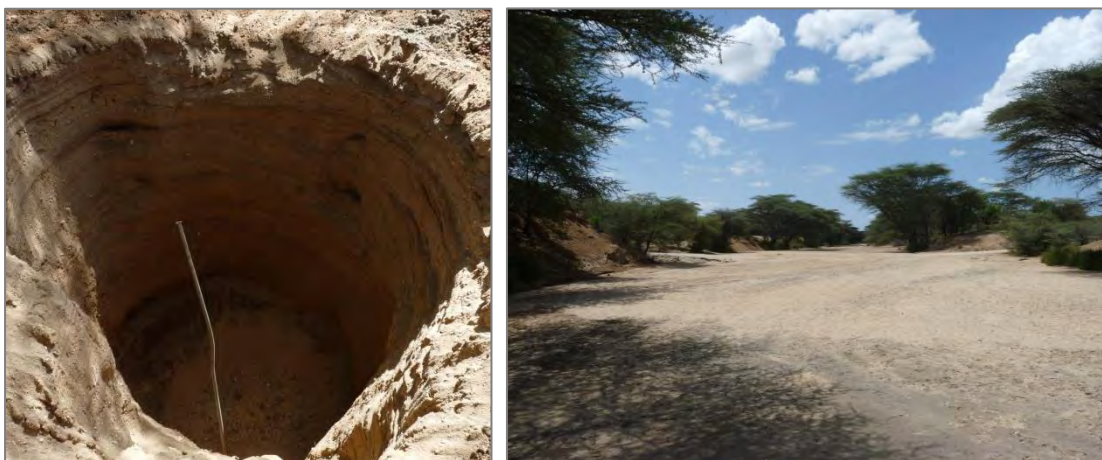
Figure 5-4: Test pit in Keekunyuk River, the dark layer at the bottom is a clay layer (left). Riverbed with sand near Nakabosan (right)
