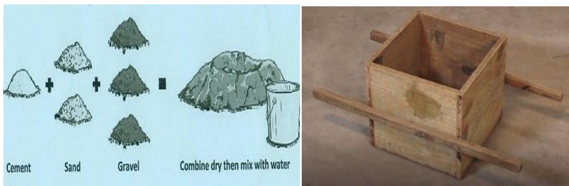
Fig-20: Mix ratio and batching box
