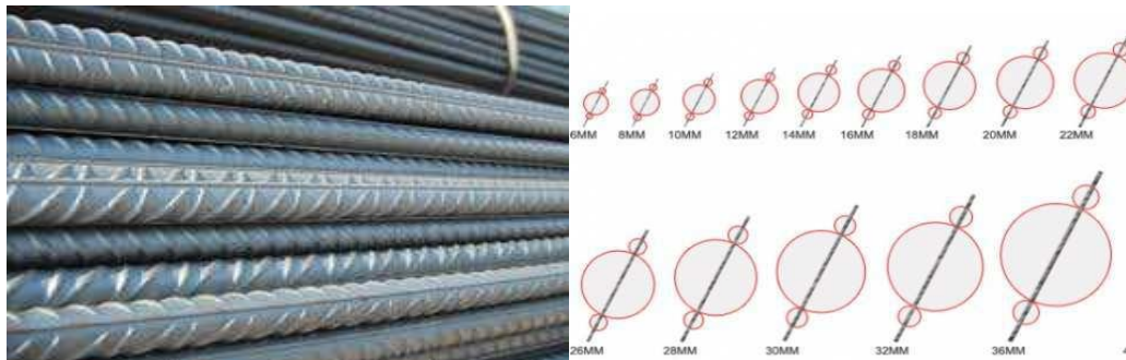
Fig-8: Rebar standard Size
