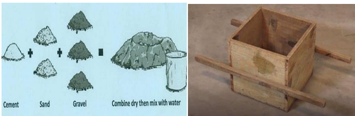
Fig-20: Mix ratio and batching box
