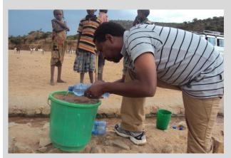
Sand and sub-surface dam design requires careful measurements such as the depth and porosity of sand. Research at this existing site included estimating the cost and storage capacity of the sand dam. At Kenchera, cost over-runs resulted from errors in measurement of depth to bed rock.
